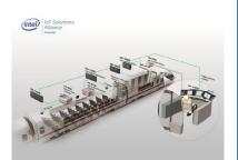
operators track and monitor train cars, with a panel PC for control. The system helps improve security and safety of passengers. Advantech Rolling Stock solutions are EN 50155 compliant with M12 connectors
